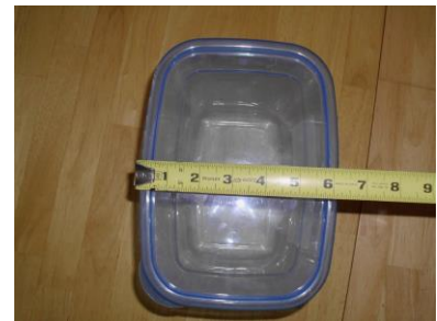
1- large reservoir or reservoir support container 8 3/4" long X 6 1/4" wide X 6 5/8" high.
