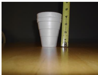
20 – Styrofoam cup “canal supports” 3 3/4" high. When stacked, each cup adds an additional 1/2" of height.
